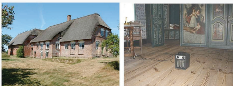
The traditional farmhouse Kommandørgården is located at the West coast of Jylland. It has conservation heating with moveable electric heaters controlled by hygrosstats.
